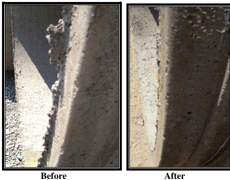
Figure 2-18. Spigot Finning Repair – Acceptable
