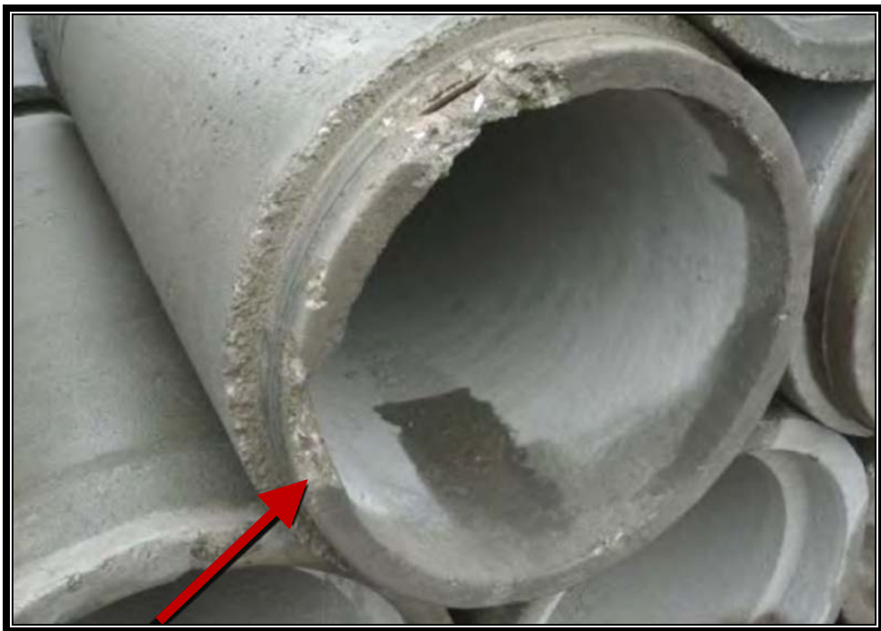
Figure 2-3. Chipped Spigot End – Repairable
