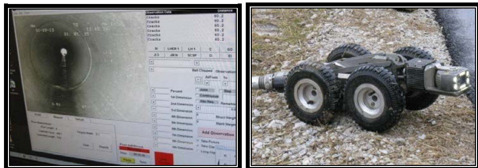
Figure 6-2. Video Inspection Equipment
