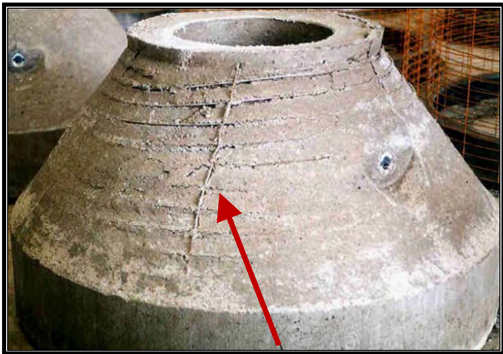
Figure 4-6. Exposed Conical Top Reinforcement – Not Acceptable
