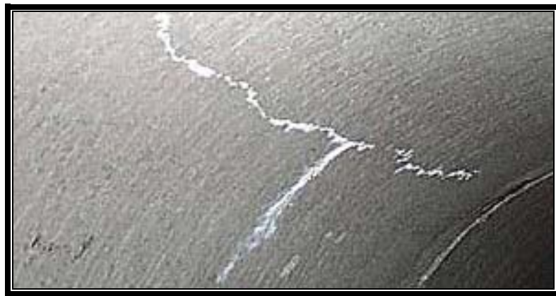
Figure 6-4. Autogenous Healing in Concrete Pipe
