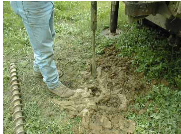
Figure 16. The shear vane is inserted into the hole and carefully pushed about 1 foot into undisturbed soil at the bottom.
