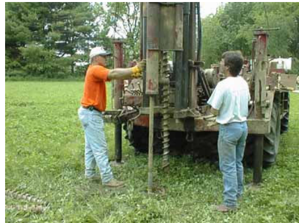
Figure 4. The SPT split-spoon sampler is placed at the bottom of the augered hole. A 140-pound automatic-trip hammer, falling freely approximately 30 inches, drives the sampler a depth of 18 inches. The driller records how many "blows" it takes to drive the sampler each 6-inch increment.
